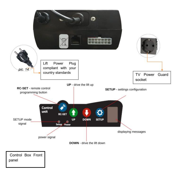
14. Connecting the controller: connect cable from the lift with the control box. Then plug in the main socket. The power supply is signalled by lighting the indicator POWER (green). Then the controller carries out the procedure "self-test" indicating this by three sound
